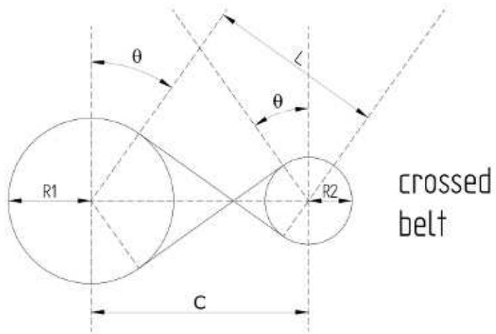
Figure 3. Crossed belt pair of pulleys.
