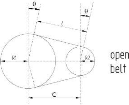
**Figure 2.** Open belt pair of pulleys.
